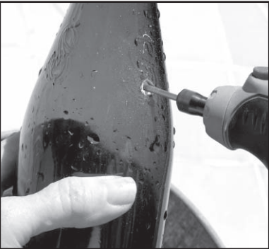
1. Drill a hole in your bottle using a glass cutting bit. (Wear safety glasses and cut over a bucket to catch glass).
